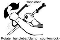
2. wise toward engine until clamp falls into groove of base.
